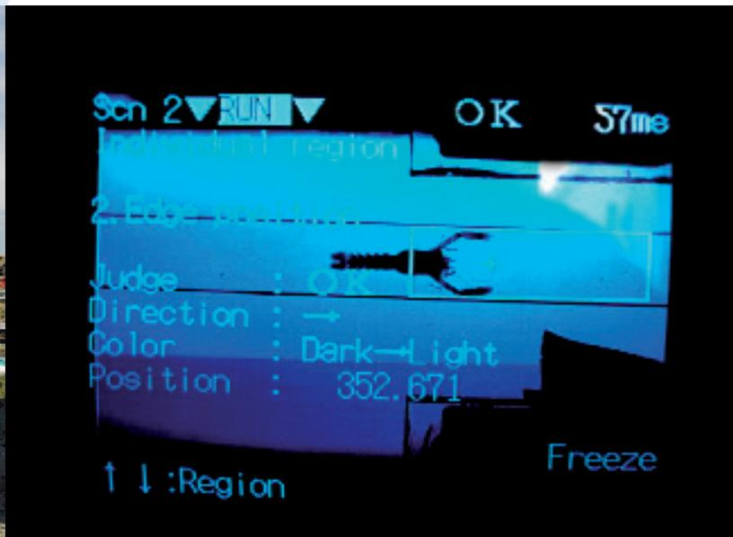
A lobster passing through the size grading robot. Photo by A. Drengstig
